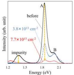
Photoluminescence (PL) for monolayer  $MoS_2$  is also measured after irradiation. It was found that PL is much more sensitive under the low irradiation dose. After the ion beam irradiation, A peak around 1.85 eV decreases and impurity peak D around 1.3 eV disappears, which indicate the non-radiative relaxation of electrons transitioning to defect level appears.
